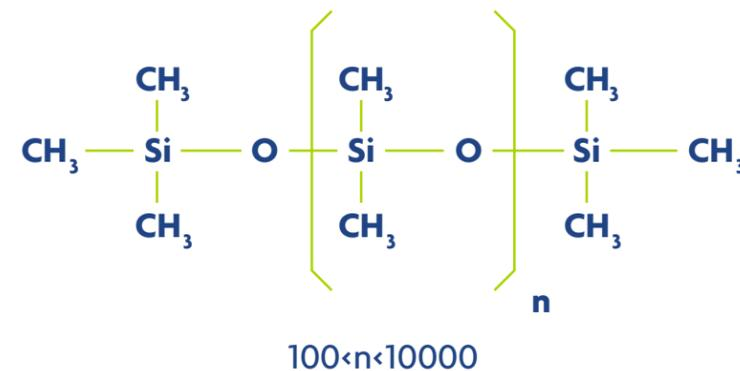
A silicone oil named polydimethylsiloxane (PDMS) and silica particles are the two major ingredients of a silicone antifoam agent.
